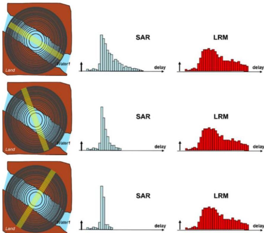
**Figure 2: Echoes in SAR or LRM modes according to the respective position of the satellite trajectory (perpendicular to the rectangles of the SAR mode) and the watercourse. Footprints are represented as orange rectangles (SAR footprints) and black concentric circles (LRM footprints). (Credit: Aviso - CNES)**
