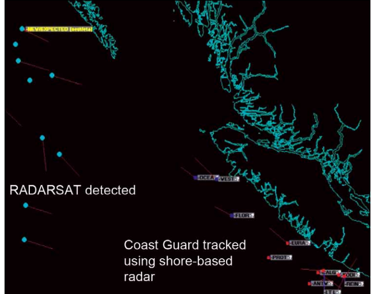
RADARSAT-2 is able to detect rogue ships far in advance of conventional shore-based radar systems, and far beyond the reach of airborne sensors.
