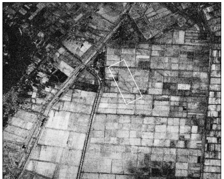
Coherence Change Detection senses surface changes to detect active routes as seen by these tracks through the fields indicated above.
